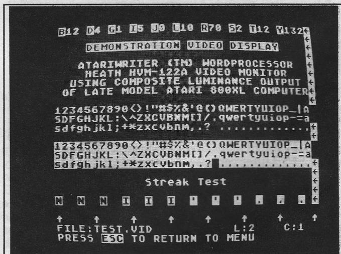
Figure 2C. Luma output of late-model (Taiwan) stock 800XL: sharpness much improved but background is still grainy. XE machines also look like this.
