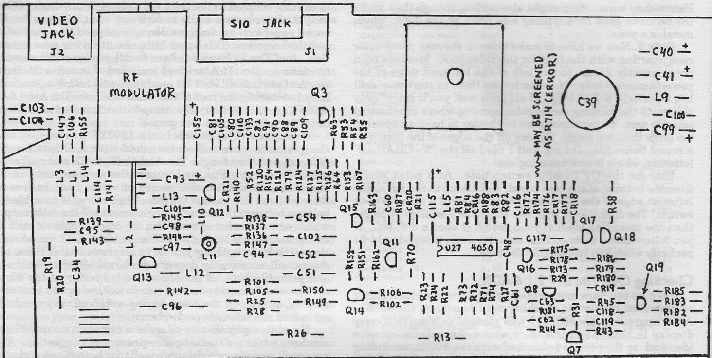
Figure 9. Parts placement diagram for the 1200XL.
