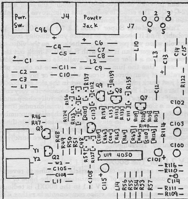
Figure 8. Parts placement for the 600XL
